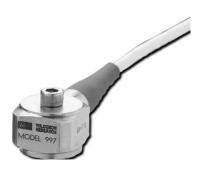
High frequency accelerometer, 10 mV/g sensitivity, ±10% sensitivity tolerance, 500 g range, low profile with side exit integral cable, ring type with 8-32 thread captive mounting screw
