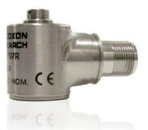
Accelerometer, radiation-resistant ( $1x10^{-7}$  RADs exposure limit), 100 mV/g sensitivity, ±5% sensitivity tolerance, low profile with side exit MIL-C-5015-style connector, case isolated
