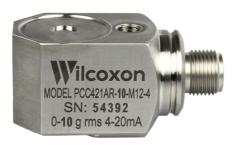
Vibration transmitter, 4-20 mA output proportional to RMS acceleration, 5 g full-scale measurement range, operation to 105°C, low profile with side exit 4-pin M12 connector, the upgraded PCC42X series is smaller, lighter and lower price
