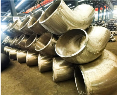
bend and Alloy elbow of P91
