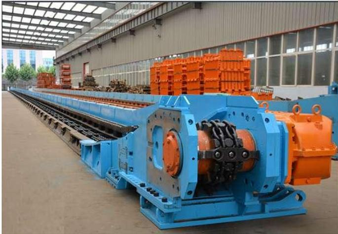
Thermal power plant Coal feeding machine customized length coal feeding machine of boiler coal transportation
